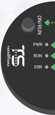
The control panel for the Brawndo TS system is operated by pressing a single button on the top of the unit.
